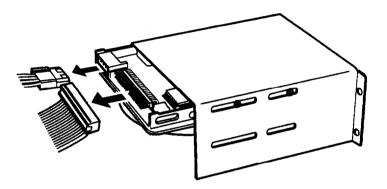
2. If you will be removing your only IDE hard disk drive, disconnect the hard disk drive ribbon cable from its connector on the main system board.
